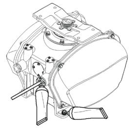
**10.** Use silicon sealant around the mounting bolts
