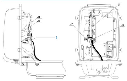
8. Use the cable clamp (1) to secure the cable to the upper housing. The clamp should hold the cable at the point where it is wrapped in copper tape.
