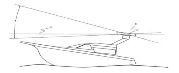
In this case, you're recommended to install the scanner so that it is tilted down at the front, at an angle that will produce an almost horizontal sweep when the power boat is running at speed.
