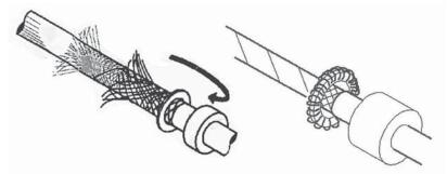
Carefully unwrap the copper tape (1) and black PVC tape (2). Shorten both the foil shield (3) and the clear insulation material (4) so that an extra 50mm of cable is exposed. Re-use the copper tape on the end of the foil, ensuring it is stuck to the same side as before, to ensure good conductivity.
