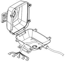
7. Connect the five scanner cable connectors to the 'J' connectors as follows:
