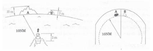
In this example, the scanner is installed on the vessel at a height of 3 m (10 ft) above sea level (h1). Island A is 10 m (33 ft) high (h2) and for comparison, island B is 5 m (16.4 ft) high (h2). Both islands are at a distance (D) of 10 nautical miles from the vessel.
